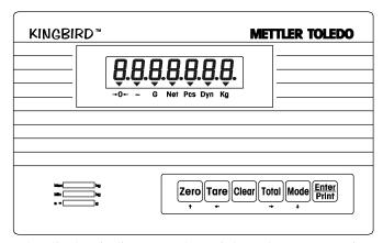
The display indicates scale weight unless you are in setup mode programming the KINGBIRD or using prompting. Error messages are displayed as they occur.
