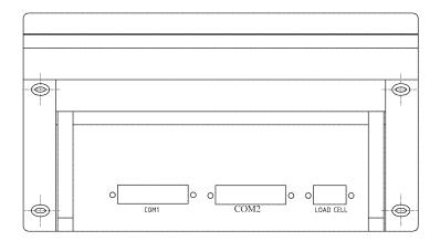
COM1: one 25 pin female D subminiature for RS232 serial port.
