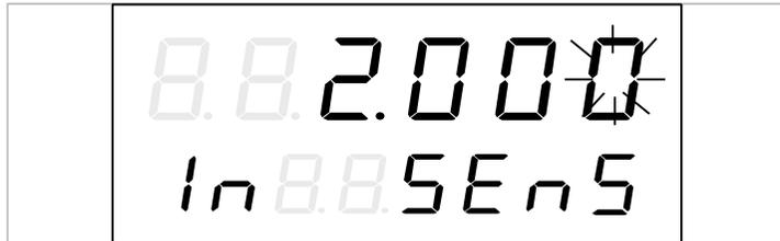
Input 'Output Sensitivity of Loadcell' [SEnS]: 0.500~5.000mV/V.
