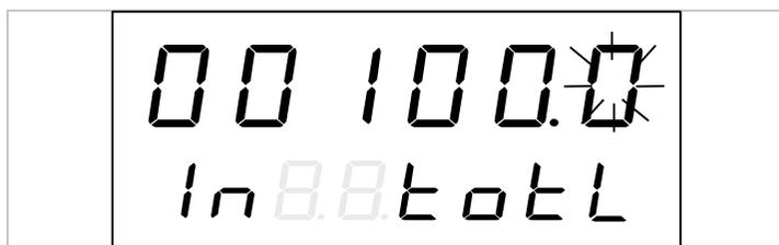
Input 'Total Capacity of Loadcells' [totL]: 1~100000kg.
