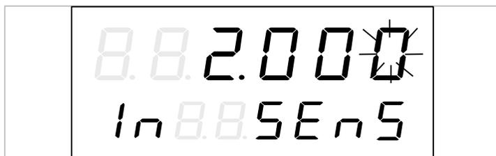
Input 'Output Sensitivity of Loadcell' [SEnS]: 0.500~5.000mV/V.
