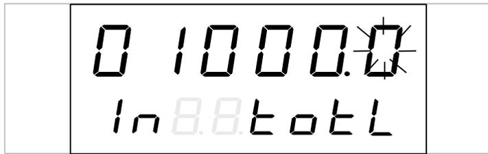
Input 'Total Capacity of Loadcells' [totL]: 1~100000 Weight Unit.
