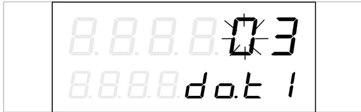
Input 'Holding Time of DO output state' [do.t]: 1~99s.
