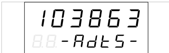
Input weighing signal 0~25mV to test linearity of AD value.
